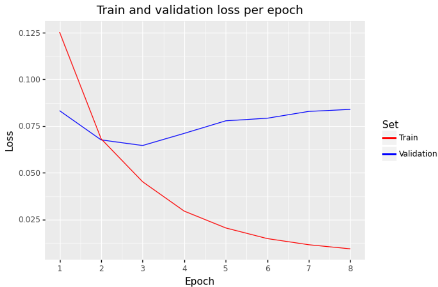
Fig. 5.2: Training set and validation set loss per epoch.
