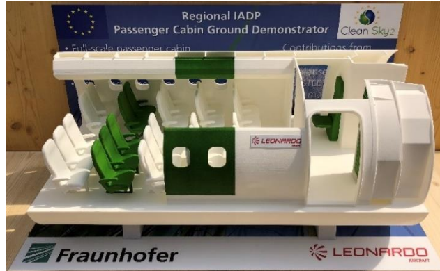
Figure 7: 3D printed model of the Passenger Cabin Ground Demonstrator
