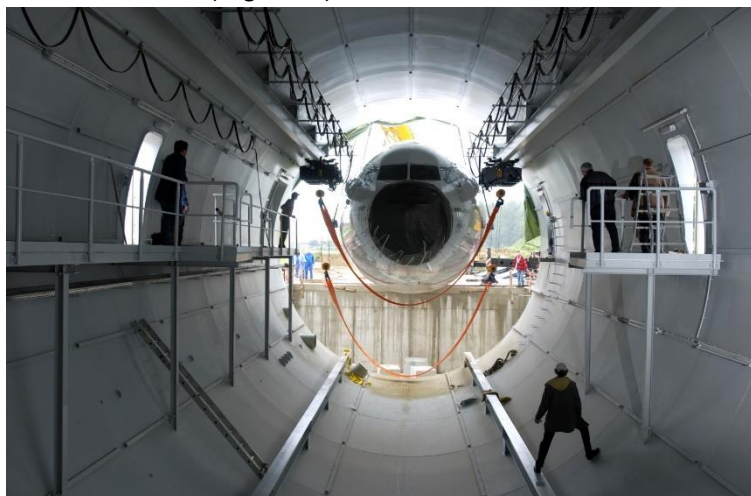
Figure 2: Fuselage integration in low pressure vessel
