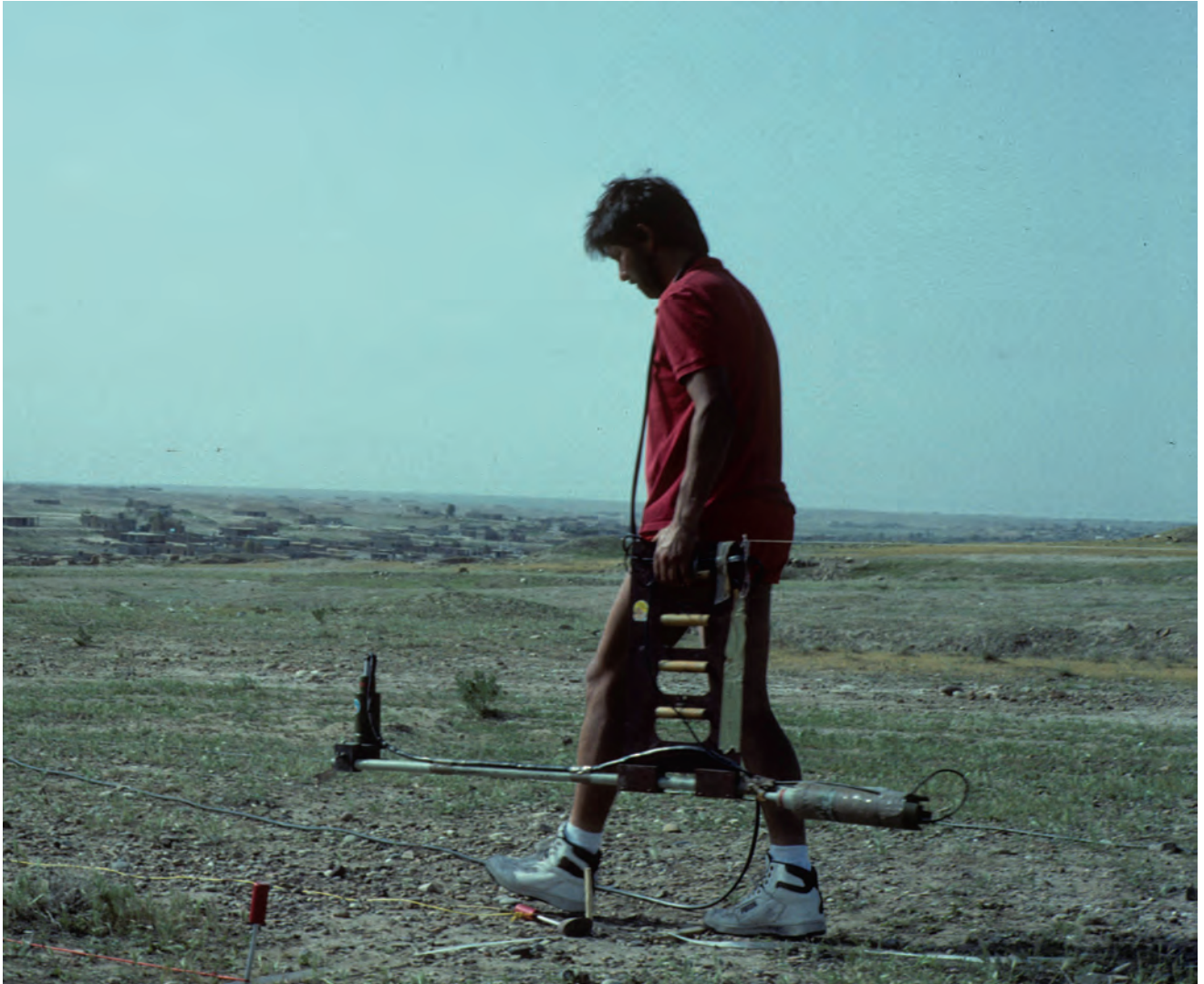
Fig. 1. Assur 1989. Magnetometer prospection with a handheld Caesium Magnetometer (Varian V101) with electronic data collection in a variometer configuration (Photo: M. Stephani).
