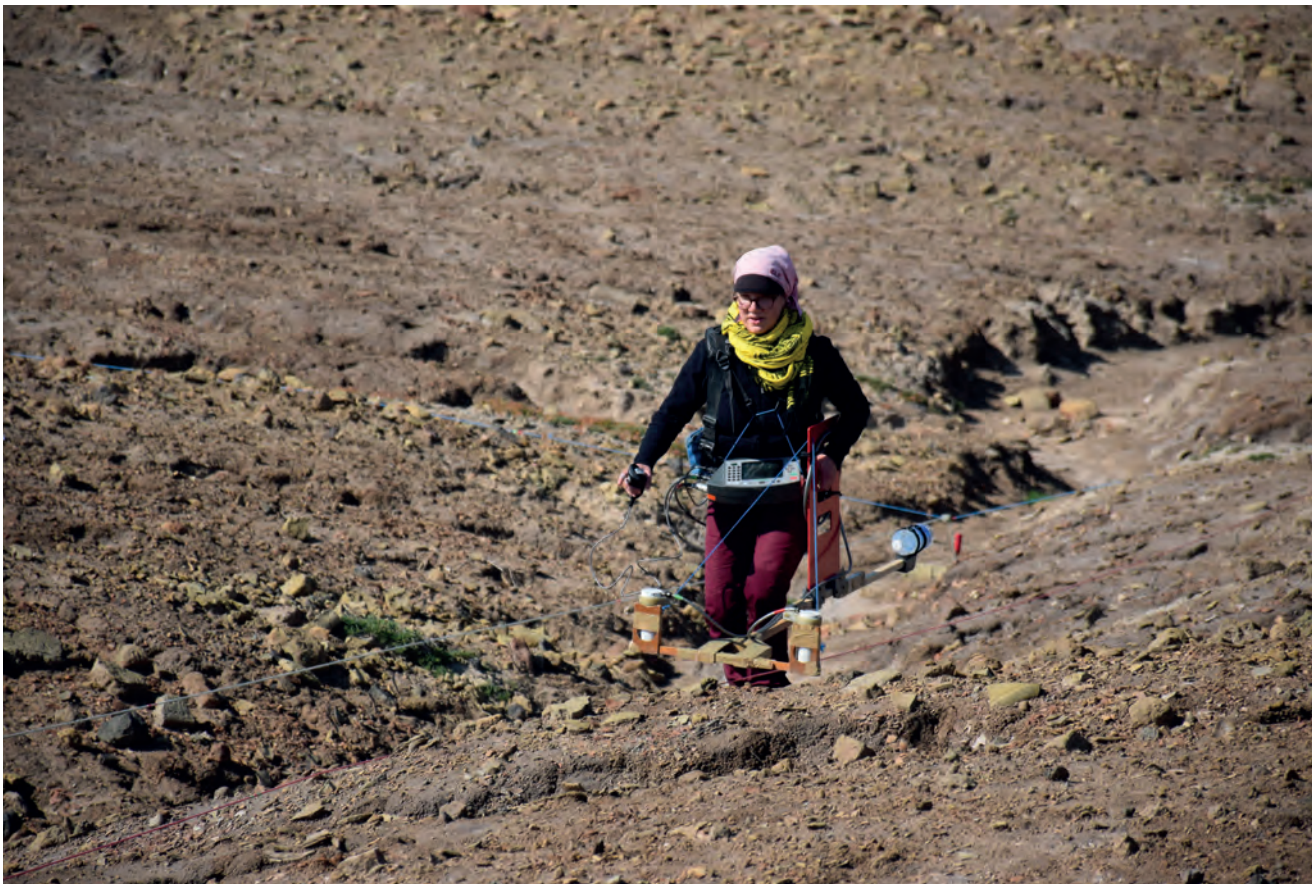
Fig. 3. Ur 2019. Magnetic prospection nowadays with the handheld total field magnetometer Geometrics G-858 (Photo: B. Einwag).
