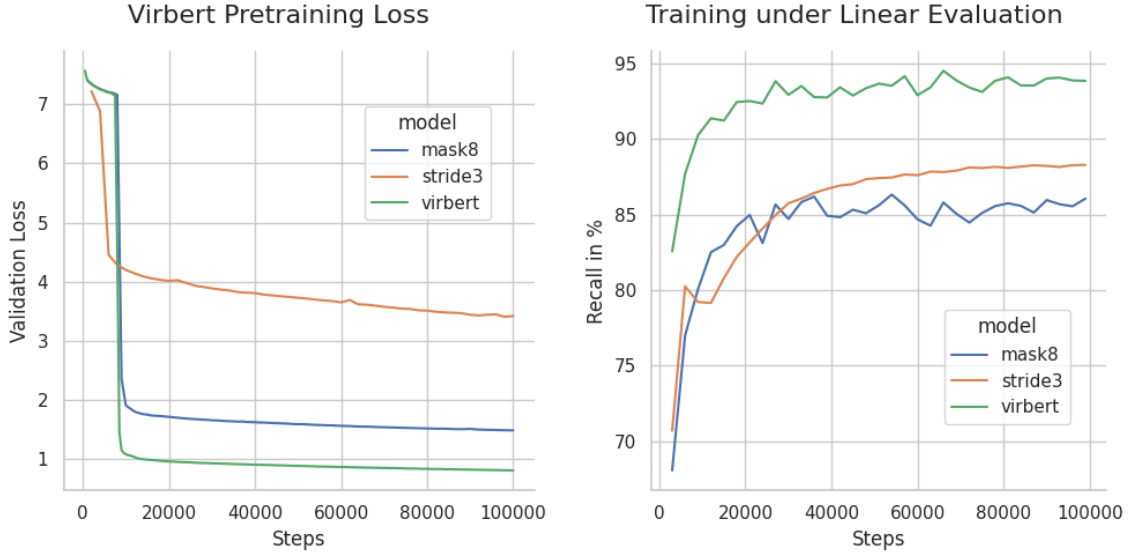
Figure 4.1: Left: Cross-entropy loss of mlm on the validation set during self-supervised pretraining of the 3 different virBERT model setups. Right: Class averaged recall during supervised finetuning of the 3 virBERT models with frozen representation model layers on the 1000nt virus phage/non-phage classification task for linear evaluation.
